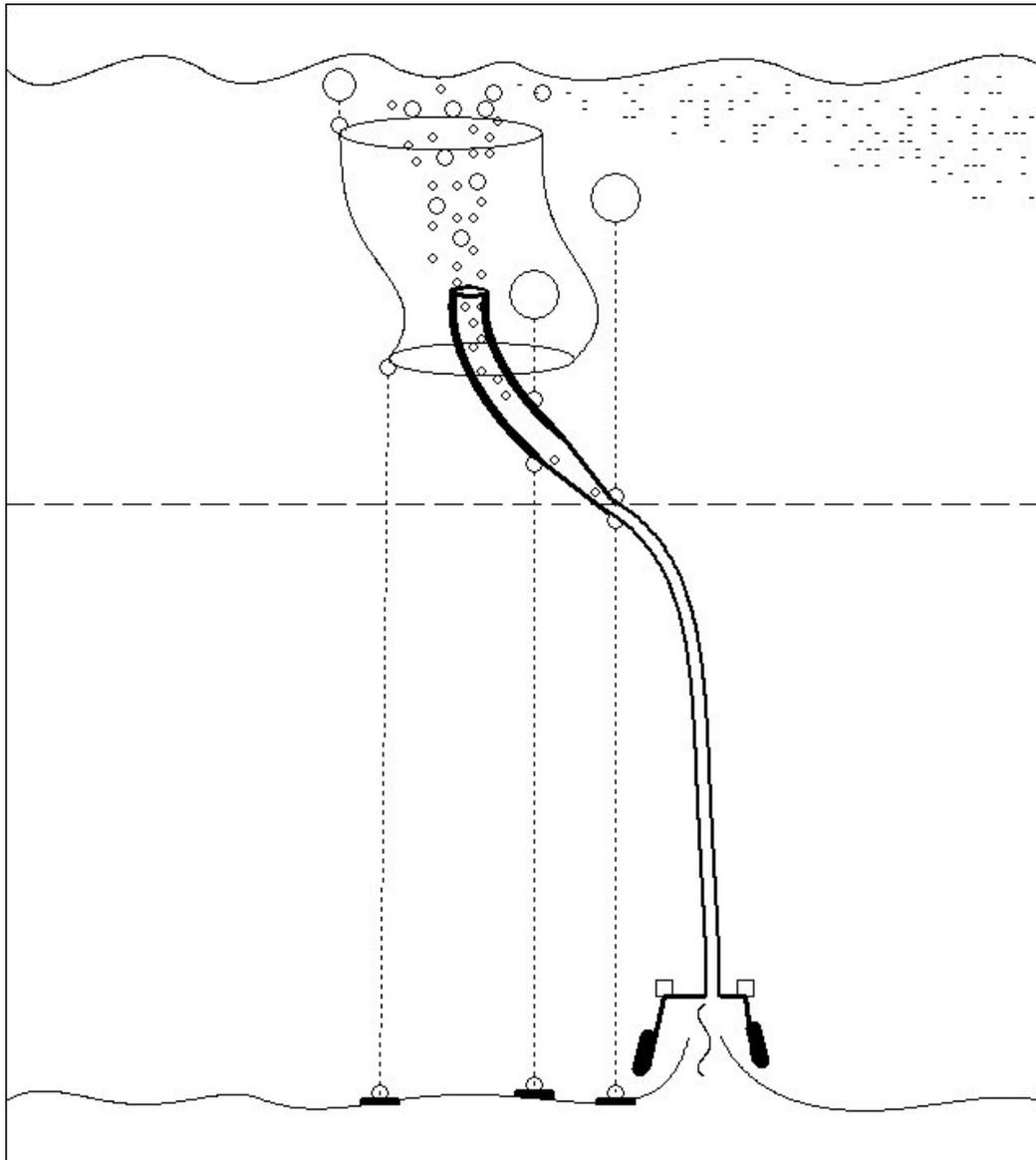
**Figure 2. A schematic diagram showing the deployment of an offshore geothermal installation in the nutrient mixing application. The upper tube is made of light weight material such as plastic film and serves to inhibit entrainment of cold water into the rising plume.**
