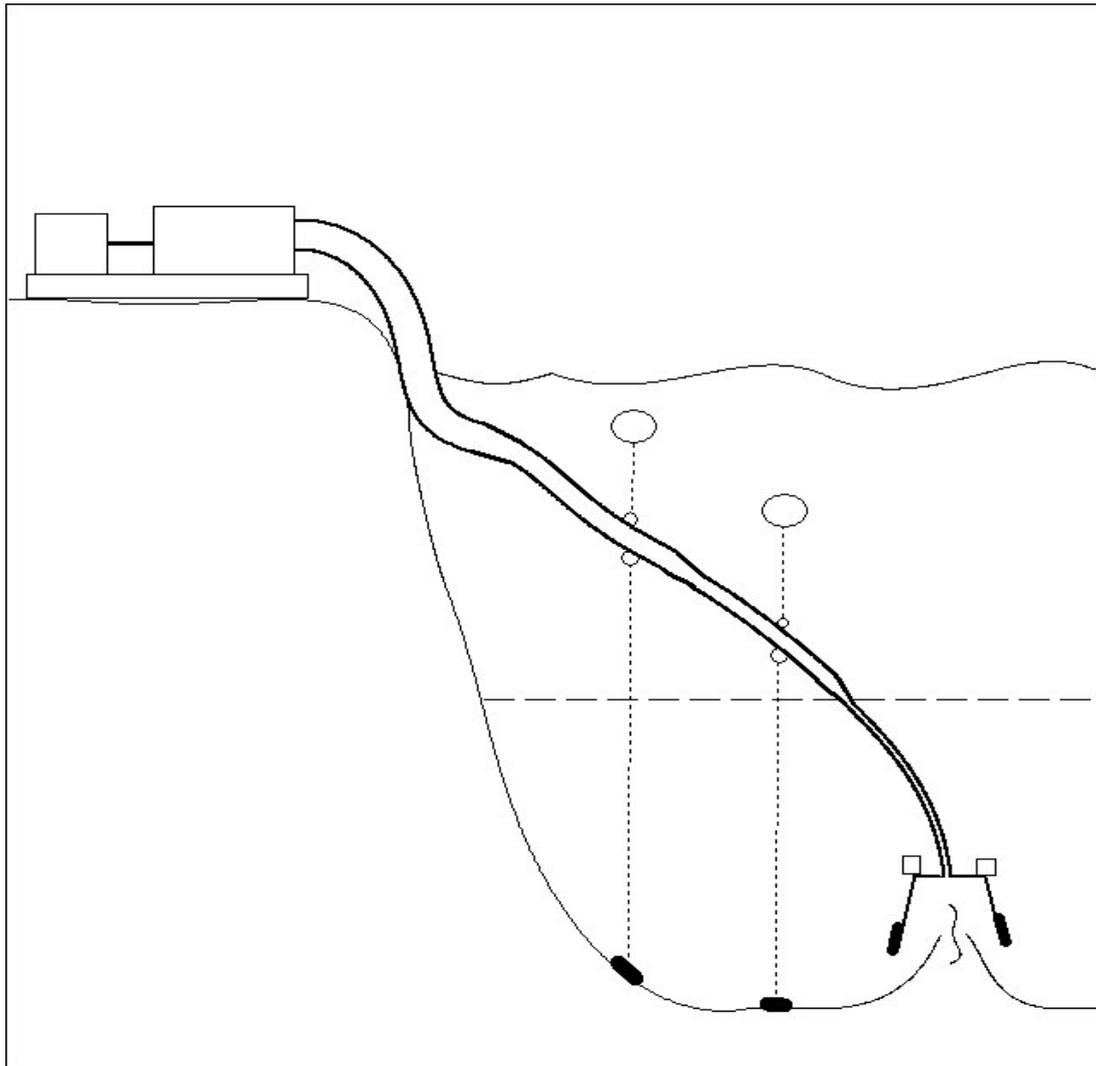
**Figure 1. A schematic diagram showing the deployment of an offshore geothermal installation in a power generating application. The insulated conduit is flared to allow for expansion of the two phase fluid with decreasing depth. The dotted line shows the depth of vaporization, i.e. the depth at which the fluid starts to expand due to boiling.**
